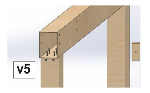
Screw the front carrier profile to the post profile with the screw V5
