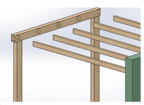
Screw to front carrier profile the falge with the screw V5
