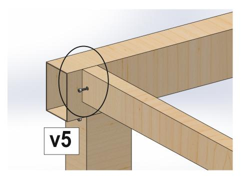
Place and screw all the carrier profile to the front profile with the screw V5
