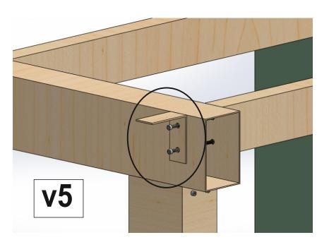
Place and install the front angle profile with V5
