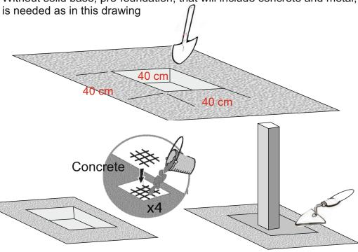
Prepare the holes of 40x40x40 cm for all the post. Make a anchorage ,and fill with concrete
