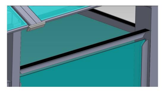
After to close all the frame cover the upper side of sheets Use a thin layers of silicon to the gap of upper profile
