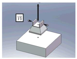
Open a hole in the floor 20 cm with bit dirl 15mm
