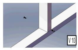
Screw from botom and up side with screw V10
