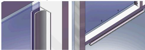
Slide the sheet on the gap of sheet profile
