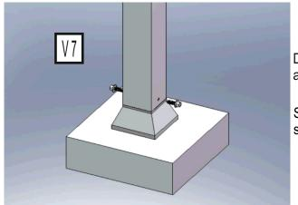
Drill with 5 drill bit the post and base
