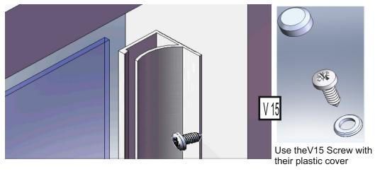
Palce the sheet profile and fix with screw V15 from one side
