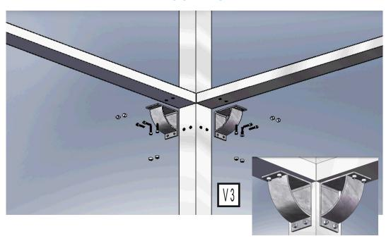
Assembly the boton sheet support profiles with the cornner part , Thight the corner part with the screw V3
