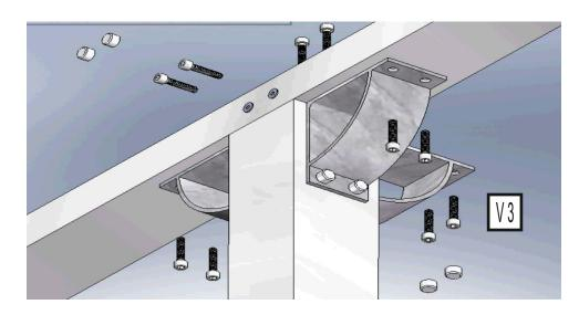
Connect the angle and post profile to the side carrier profile with the screw V3
