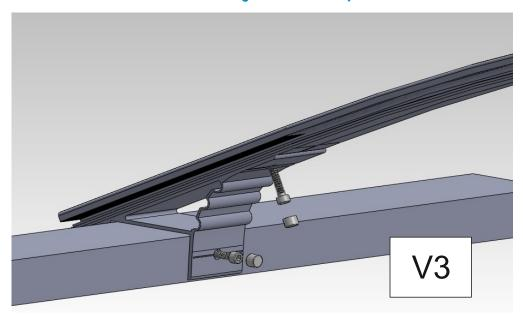
Connect with screw V3 fittings on both sides of the roof profile
