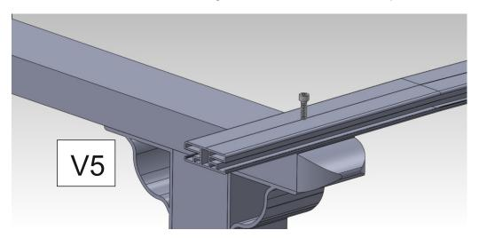
Connect with screw V5 the roof profile to the carrier pofile
