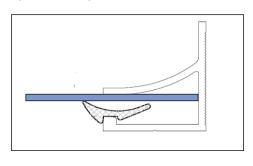
After to complit the sheet frame, Place the compression seal by squeezing it between the profile and the roof panel.
